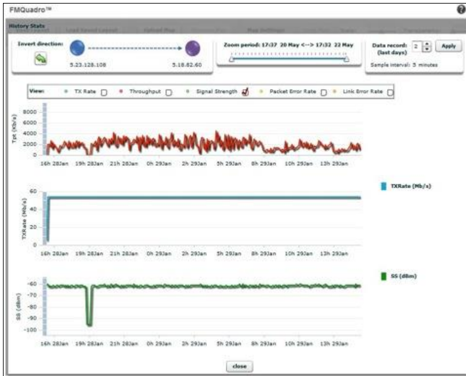
Figure 7.13: FMQuadro, Last 48 Hours Link information
