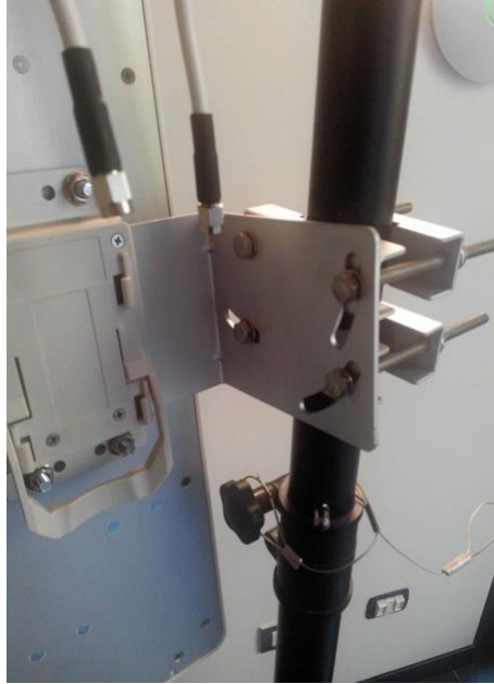
Figure 3.2: Fluidmesh 3200 Pole Mounting Adapter Proper Installation Procedures
